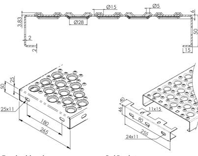
**Stair Treads with ends** Feature a folded end for fixing the Stair Tread to stringers.
